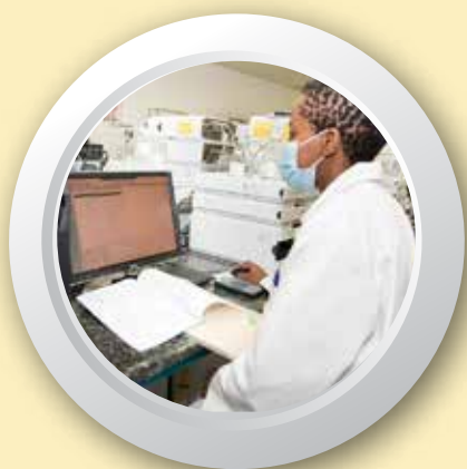
Figure 6 – HPLC units are connected to a computerised system that controls the process flow of the samples.
